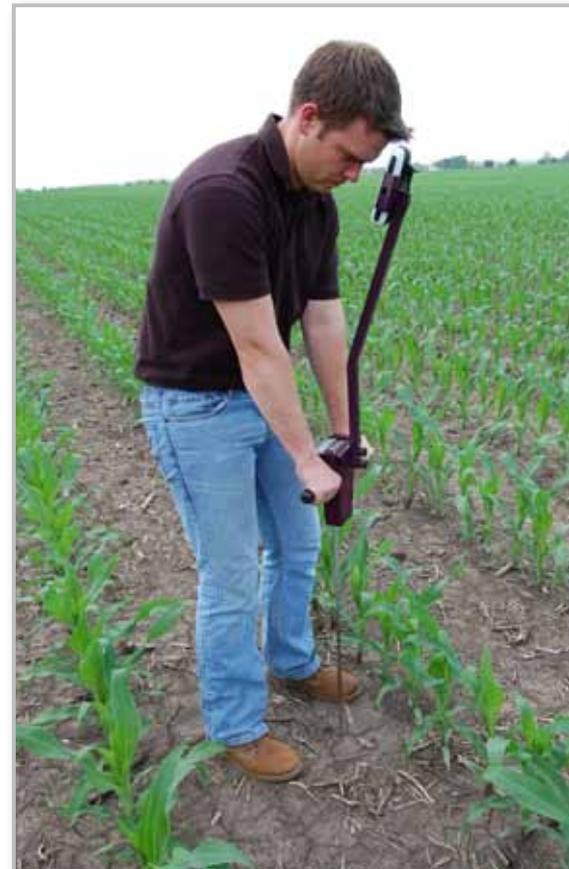
FieldScout SC 900 with GPS Unit Mounting Bracket
