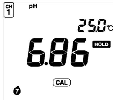
The measured value will be displayed, and “ HOLD ” will blink until the reading stabilizes.
